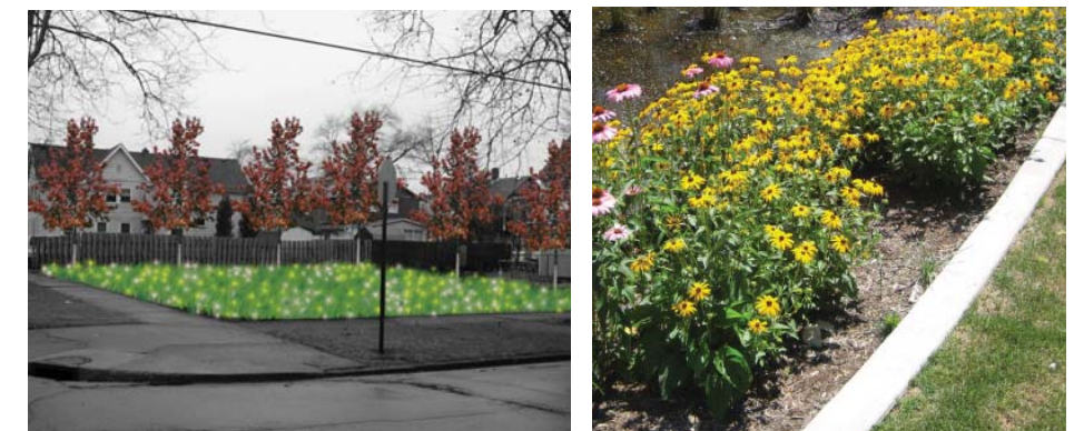
By inserting raingardens into vacant lots, runoff can be stopped before entering the CSO.
